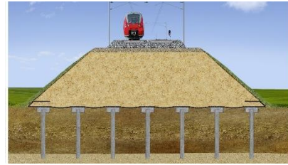
Deep Foundations on Piles
