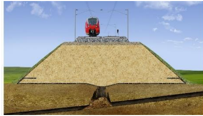
Bridging of Sinkholes
