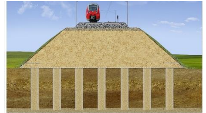
Geotextile Encased Columns
