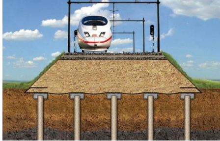
Basal Reinforcement for Piled Embankments
