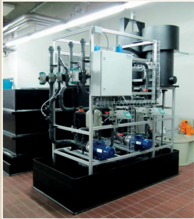
BWS separation plant for water containing oil
