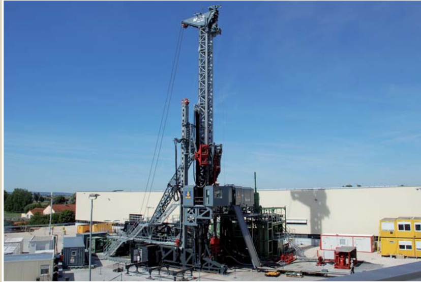
Newly developed deep drilling rigs – the TBA 300
